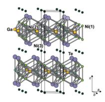
The NiAs-derivative crystal structure of mixed tellurides  $Ni_{3-x}GaTe_2$  ( $0 \le x \le 0.65$ ) hosts a variable content of Ni atoms in 2D heterometallic Ni/Ga slabs and Teconfined van der Waals gaps. At low values of Ni content, x < 0.5, the extra Ni atoms arrange in a superstructural ordered fashion aimed to relax the structural strain between the occupied and vacant sites in the ab plane.
