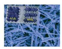
0D-1D BaTiO<sub>3</sub> nanostructures with perovskite structure were synthesized by using  $H_2Ti_3O_7$  nanowire templates under low-temperature (80 °C) solvothermal conditions in an ethanol/water mixed solution.
